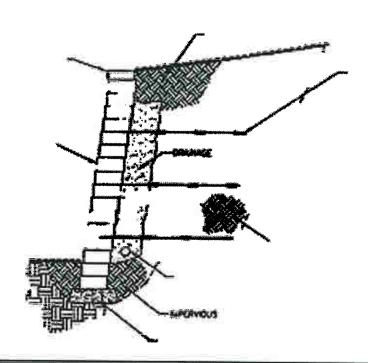
Section of retaining wall to be built behind house near south lot line, 23 feet in length. The wall will be terraced, with two steps of four feet each. Shrubs and flowers will be planted in front of each tier of the wall along with hanging vines to complete the landscaping around and in front of the wall.
