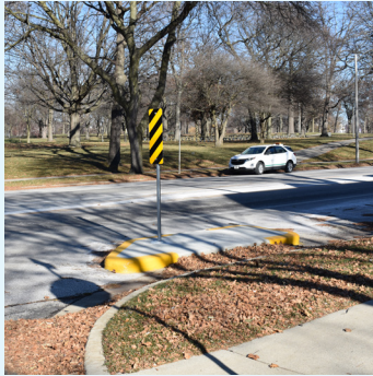
Curb Extension, Pinned-on
