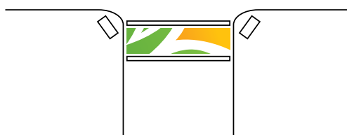
No: crosswalk does not connect two angled (Type II) ramps
