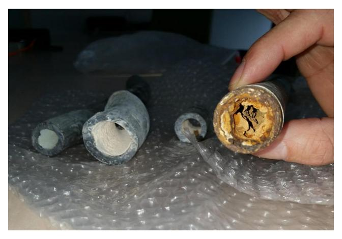
Food-grade phosphate, typically referred to as ortho-phosphate, is mixed into the water at the purification plants. The phosphate coats the pipes to prevent corrosion, or leaching, of lead from pipes and plumbing fixtures. The Milwaukee Water Works has been providing this corrosion control since 1996.
