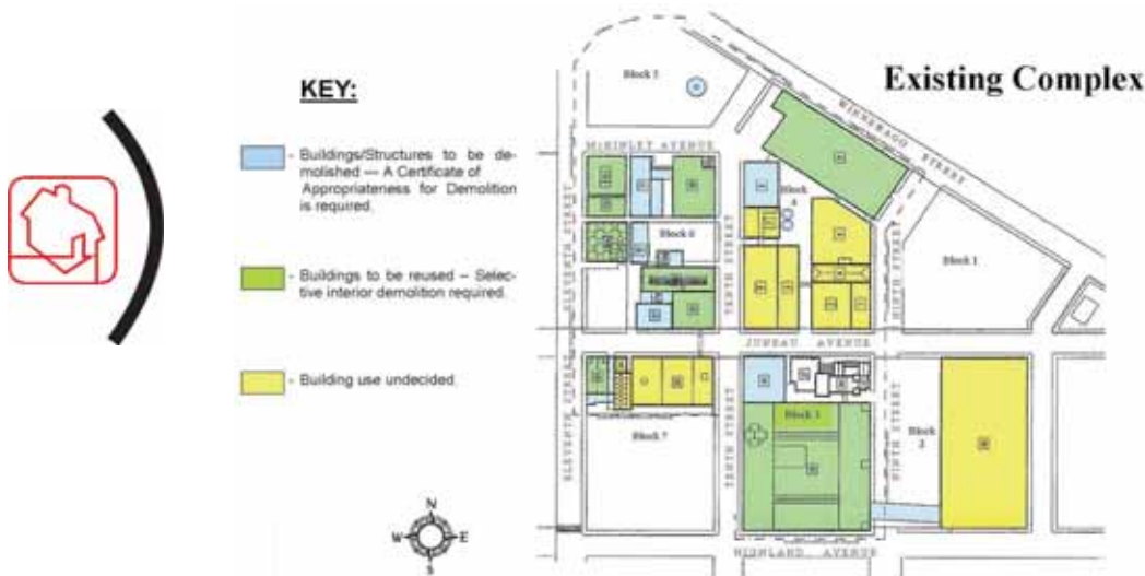
Brewery Project LLC Demolition Abatement Plan, Phase 1
